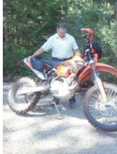
3337 Sidestand deployed. Pull bike toward you. Wheels off the ground, bike is easy to spin
