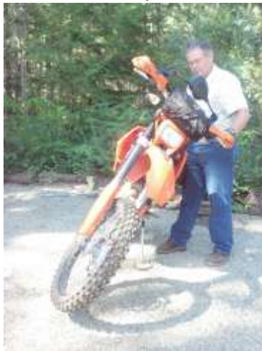
3337 Sidestand deployed. Pull bike toward you. Wheels off the ground, bike is easy to spin
